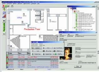
there are cardholders. Using this feature virtually means that there are unlimited access levels in the system with EACH cardholder having as many as 38 independent access levels assignment.
