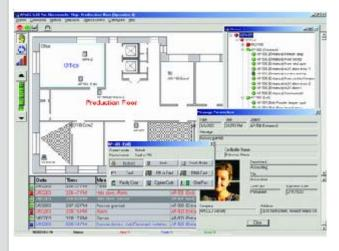
The APACS PRO program supports configuration of all field devices, access levels and time zones. These parameters are downloaded to the AANs, or the downloadable AIMs over the communication link. Additional user defined database fields can be entered by the user to provide supplemental cardholder information.
